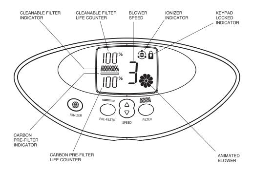
Fig. 4 - Air Purifier Control Area and Alpha-numeric Display
